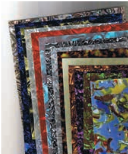
Fig 2. Cellulose Acetate in sheet form - showing the colour and effect possibilities
